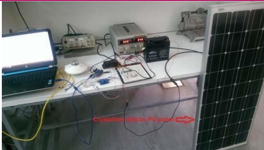
Figure 9 Laboratory Setup Including the Solar Panel
